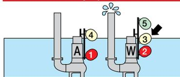
1. Float 3 operates, and pump W starts to discharge water.
