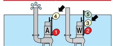
1. Start float 4 of pump A operates to start water discharge. The pump ends primary operation, and stops operating.
