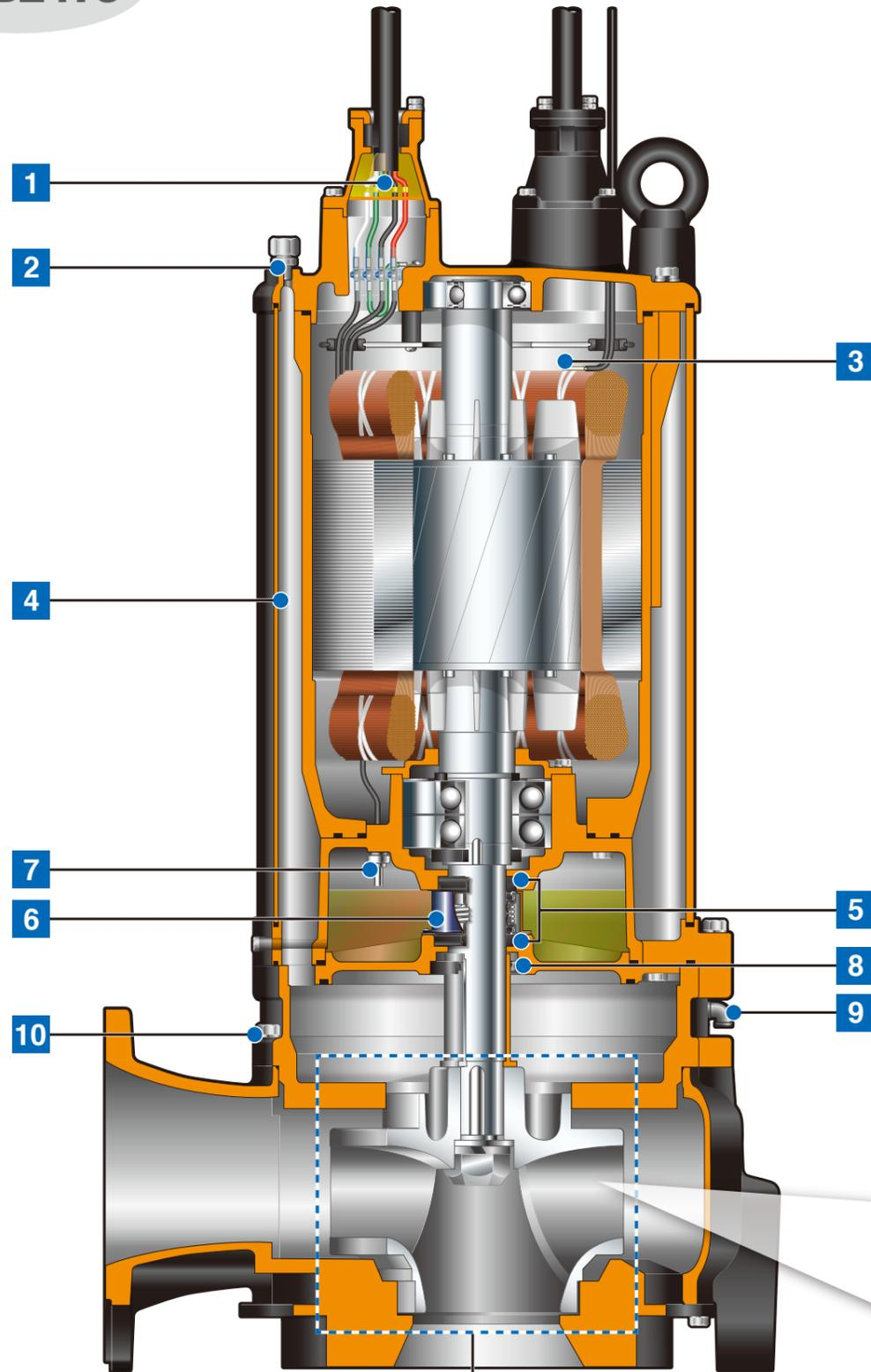
**Shrouded Channel Impeller with Wide Passages to Prevent Clogging**
