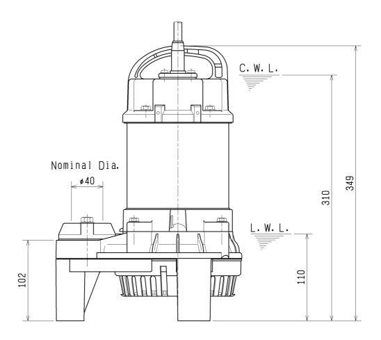
C. W. L. :Continuous running Water Level L. W. L. :Lowest running Water Level
